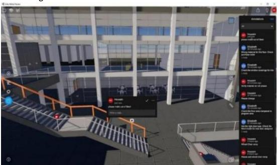
(The picture shows the modification of BIM building model with Unity Reflect in real time)
